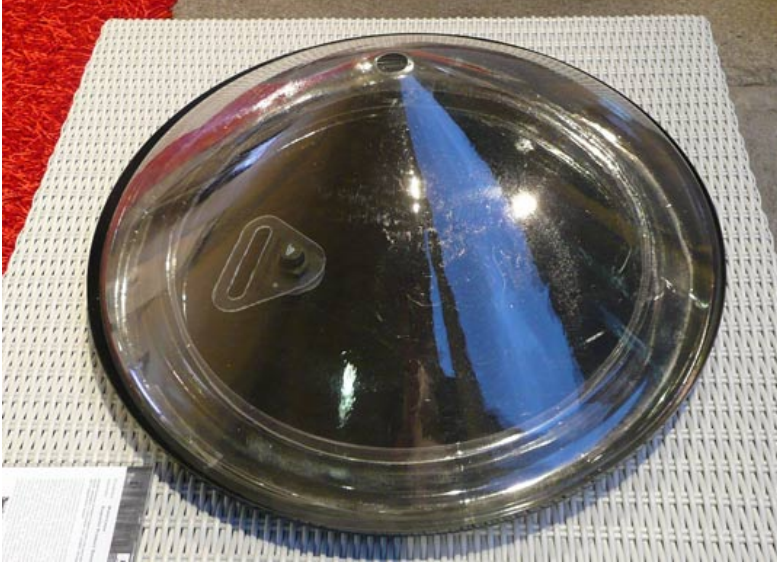
The Watercone is an cheap, mobile, and self-contained solar still that uses the principle of water condensation to render sea water and brackish water potable.
