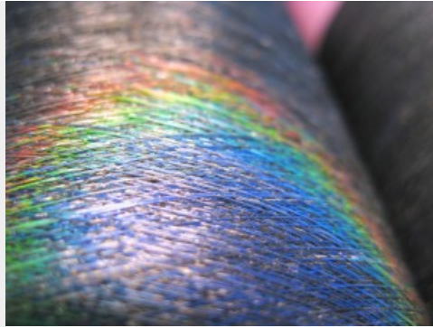
The fibres change colour when exposed to heat (photo: Louise van der Werff, CSIRO)
