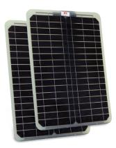
The solar panels turn sunlight into electricity. The electricity is used to charge the main battery in the Solar Suitcase. The solar panel for the Solar Suitcase is sized so that the battery can fully charge every day.
