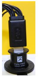
The Solar Suitcase can charge most cell phones by placing the USB adapter into the **Appliance Connector** and attaching the universal phone charger. You can also charge phones that have a 12V DC car charger. Simply plug the phone car charger into the **Appliance Connector**. Make sure the appliance plug is inserted ful-
