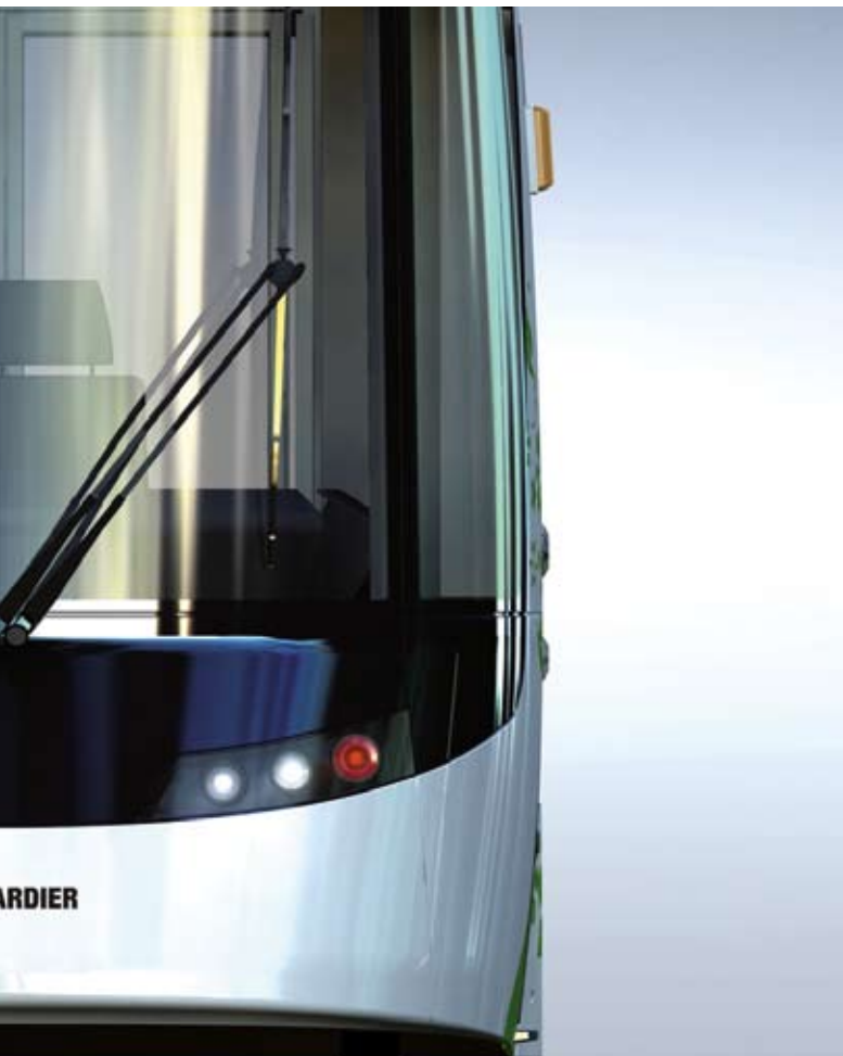
LED lighting: Used whenever it makes sense to increase energy efficiency and a lamp's working life
