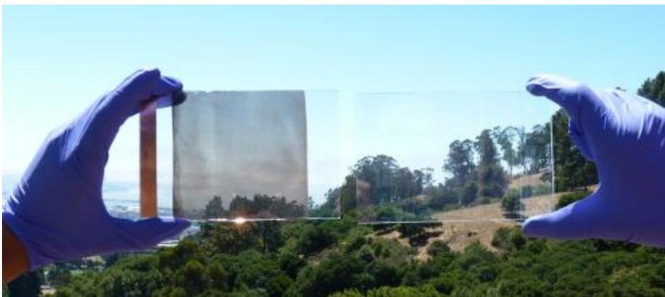
A dual-band electrochromic material has been developed by linking tin-doped indium oxide nanocrystals to an amorphous niobium oxide matrix. These transparent films are capable of blocking solar radiation in a controlled fashion, allowing daylight and solar heat to be selectively and dynamically modulated through windows. Credit: Anna LlordÀs, Lawrence Berkeley National Lab.
